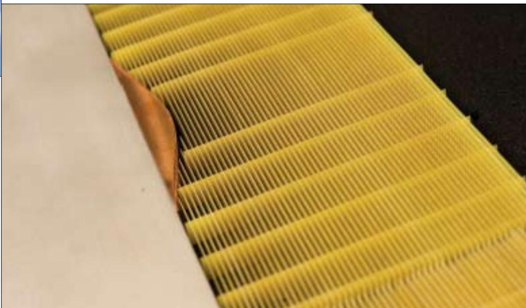
Above: John Pendry of Imperial College London. Right: A prototype invisibility device created by David Smith’s team at Duke. When microwaves shine through the meshlike metamaterial onto the copper-colored bump at center, the waves reflect back as if the bump were not there.
